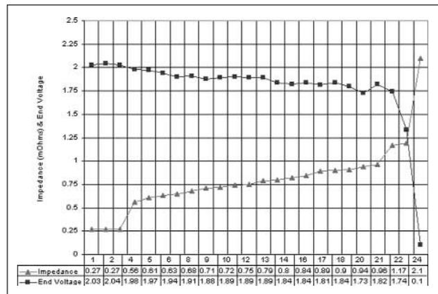
Figure 4. Ascending impedance compared to load test
