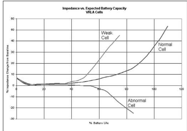
Figure 2. Impedance increases with battery age (and weakness).
