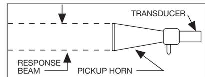
The ultrasonic transducer in the probe responds primarily to a 35- to 45-kHz bandwidth—a range found most useful for the tests described here. The transducer is very insensitive to audible sounds, allowing use of the detection system in areas with high audible background noise levels.
