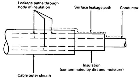
**Current Leakage Paths in a Cable**
