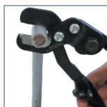
Hand-force optimised through grip adjustment
