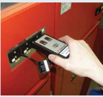
DEHNcap/IT interface test unit allows for maintenance tests at coupling units of switchgear installations according to EN/IEC 61243-5 (DIN VDE 0682 Part 415).
