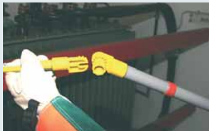
The universal gear coupling permits fast replacement of operating heads and extension elements.
