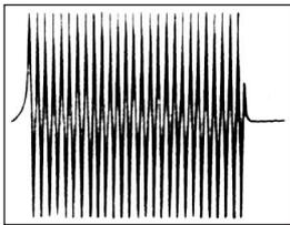
**Figure 2:** With an impedance compensation network, a recloser with a 50 ampere coil and an initial test current of 210 amperes operated in 0.783 of a second with no significant current decay. The result was well within the manufacturer's specifications.
