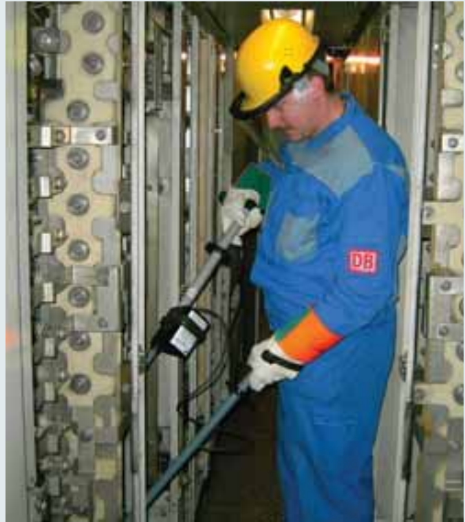
PHE/G II d.c. voltage detector for d.c. links (ICE operating head).
