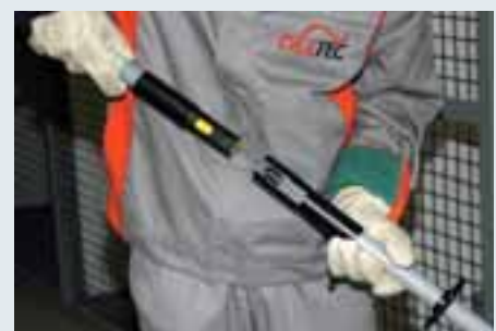
Plugging extension handle type HV STK into insulating rod type IS PHE STK.
