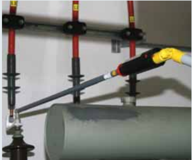
PHE III electronic indicator with universal gear coupling and insulating rod.
