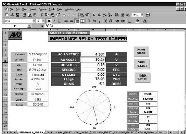
Shown above is a Test Screen for an Impedance Relay. The test result is for a Reach Test on a Impedance relay. The relay operated at 6.1 Ohms at a max torque angle of 75.8 degrees. The SR-98 software operates with Windows Excel version 7.0 or higher running under Windows 95/98/2000/NT or XP. Microsoft Excel, Microsoft Word, Windows 95, Windows 98, Windows 2000, NT or XP are all registered trademarks of Microsoft Corporation.
