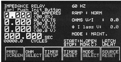
In this example, not only does the display screen show metered values, but it also displays the OHMS value where the relay picks up
