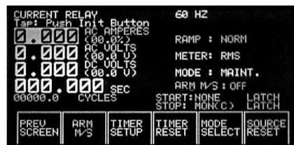
This test screen is also used to do pick-up and timing tests on current differential relays. Two SR-98 units may be used together to perform slope and 2<sup>nd</sup>, 3<sup>rd</sup> or 5<sup>th</sup> harmonic restraint tests, (\*) see Interface Port.
